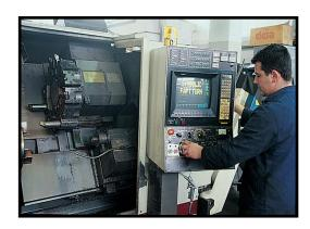
control FANUC 10 T axis: horizontal X = mm 250 transversal Z = mm 820
